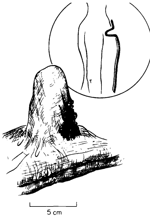
FIG. 2—Schematic drawing illustrating the cone-shaped deformation of the vest produced by a high-energy missile. Insert depicts the approximate site and size in proportion to the chest wall.
