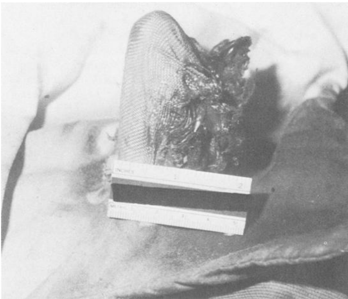
FIG. 4—The cone-shaped deformation of the vest.
